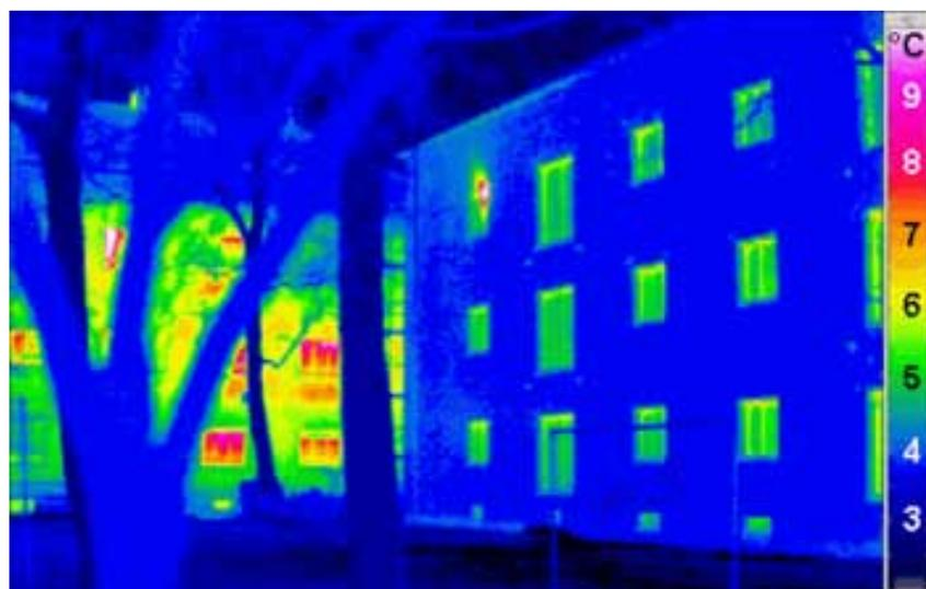
Thermal image showing house built to energy efficient PassivHaus standard in foreground and conventionally built house in background. Photo courtesy Passivhaus Institut, Germany
